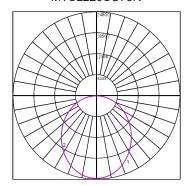
Maximum Candela = 24853 Located At Horizontal Angle = 0, Vertical Angle = 0 #1 – Vertical Plane Through Horizontal Angles (90 - 270) #2 – Vertical Plane Through Horizontal Angles (180 - 0)
