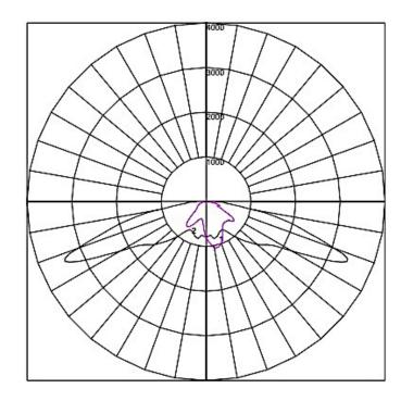
Maximum Candela = 7964.91 Located At Horizontal Angle = 75, Vertical Angle = 70 # 1 - Vertical Plane Through Horizontal Angles (90 - 270) # 2 - Vertical Plane Through Horizontal Angles (180 - 0)
